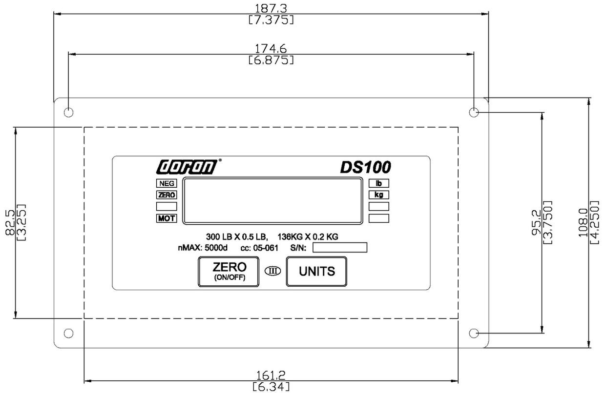
The cutout required for remote switch installation is 2.0" wide by 1.8" high. The minimum depth required for the main and remote display is 1 3/4" plus an additional 2.0" for the cable. The display is mounted by four #6 wood screws with a 90 degree countersink.
