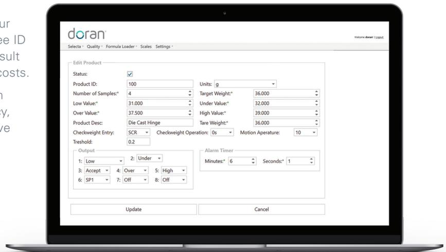
Setup screen allows for fast entry of weighing parameters and controls for each 2200CW checkweigher or for multiple checkweighers.
